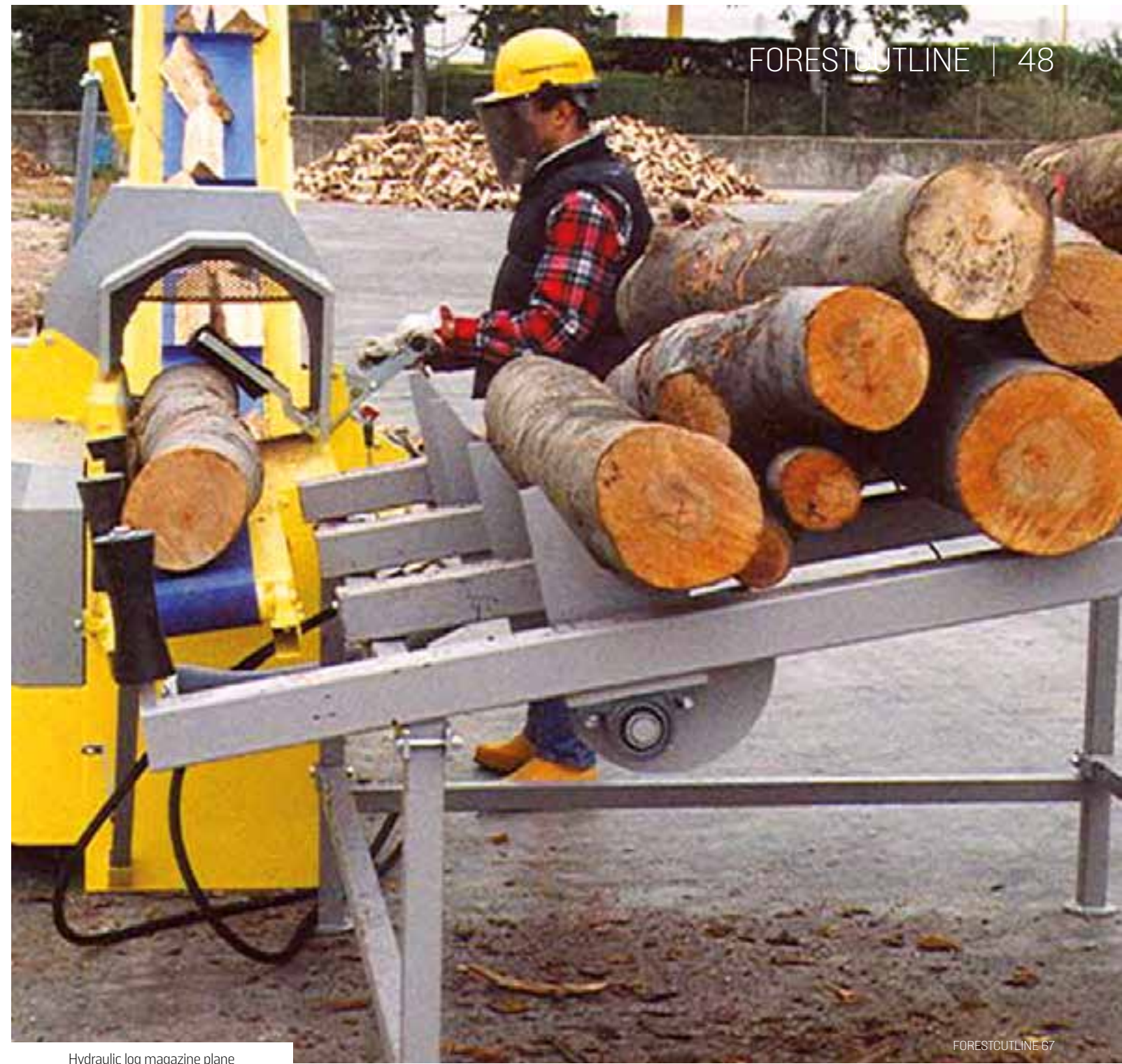
Hydraulic log magazine plane
