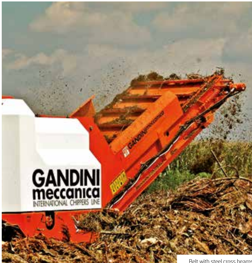
Belt with steel cross beams
