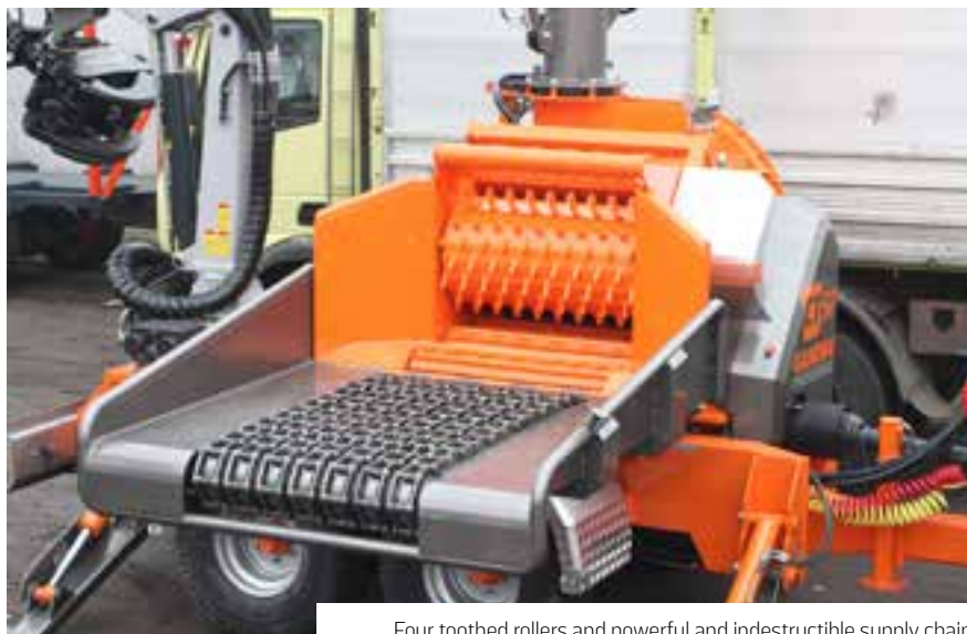
Four toothed rollers and powerful and indestructible supply chain
