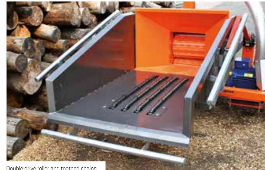
Double drive roller and toothed chains
