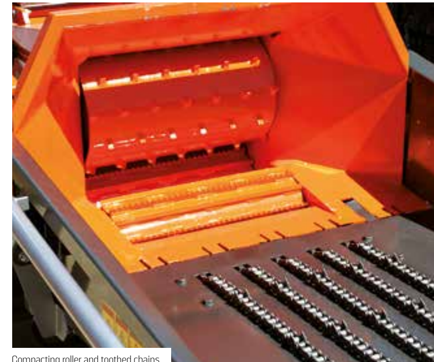
Compacting roller and toothed chains
